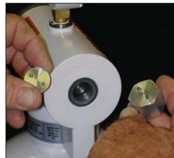
FIGURE 2. Remove security cap with the spanner tool.
