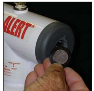
FIGURE 3. Remove the vent screen.
