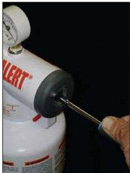
FIGURE 5. Lock open the piston.
