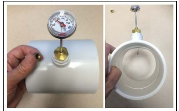
Temperature Port (Shown with Probe)
